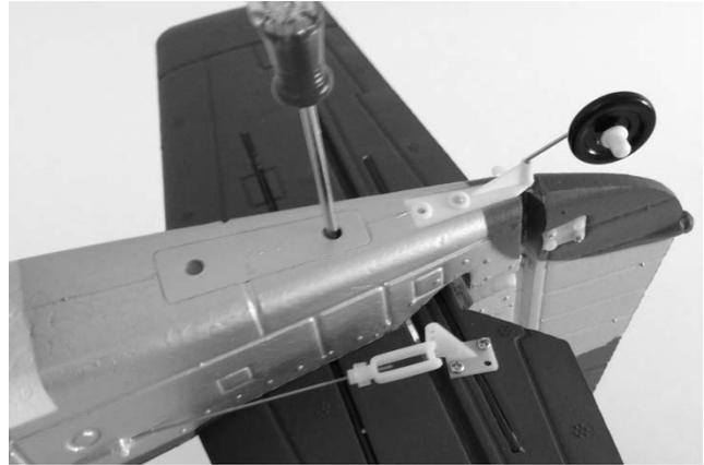
The horizontal tail/stabilizer is now installed, and please be sure to proceed through the following sections of the instruction manual (starting on page 16) before attaching the clevises to the rudder and elevator control horns.
